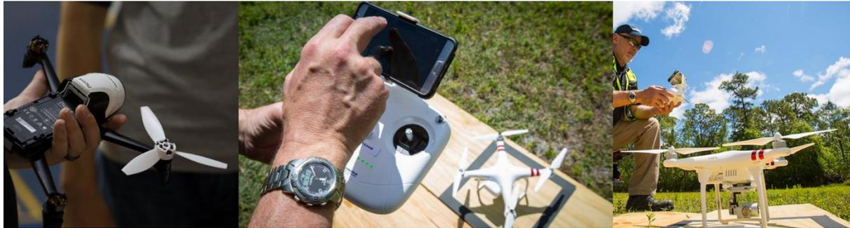
**Fig. 1: Pre-flight inspections of sUAS**
